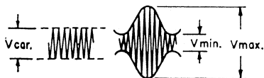
Figure 103. The amplitude modulated wave; V_{car} is the amplitude of carrier before modulation.
